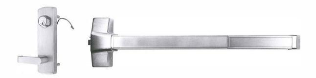
This electrically controlled lever trim provides remote means of locking and unlocking the outside lever handle. It is used with our mechanical Rim SVR CVR exit devices on non-fire rated and fire rated egress doors. Operation of the outside digital keypad will allow to lock or unlock the trim capabilities. When a correct code is entered into the keypad, electrical power will either be applied or removed to the trim, making the lever active and allowing ingress.
