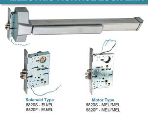
The Electric Mortise Lock Exit Device functions like a standard mortise lock but adds electronic control of the outside trim via a customer-supplied switching device (e.g., key switch, keypad, card reader, or console). The key cylinder provides mechanical override when electrically locked.
