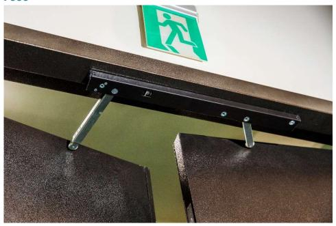
The 7600 Universal Door Coordinator is designed for pairs of doors up to 8' (2438mm) wide. It provides a smooth, quiet, and functional means of controlling the closing sequence of active and inactive doors.
